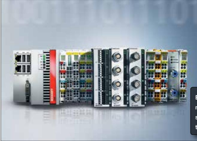
EtherCAT measurement modules, including the new ELM314x Economy line, can be used to seamlessly integrate high-end measurement technology into control systems.
